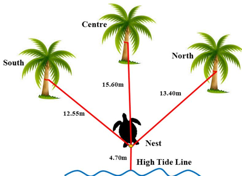
**Fig 3:** An example of the nest triangulation, to mark the nest location. The red lines indicate the measurements taken from the egg chamber to the three fixed points in the vegetation.
